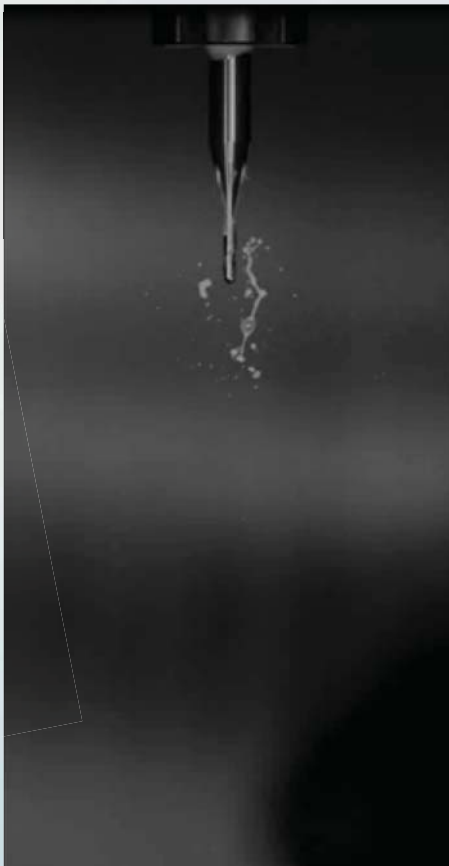
Switching on GuhroJet internal cooling
